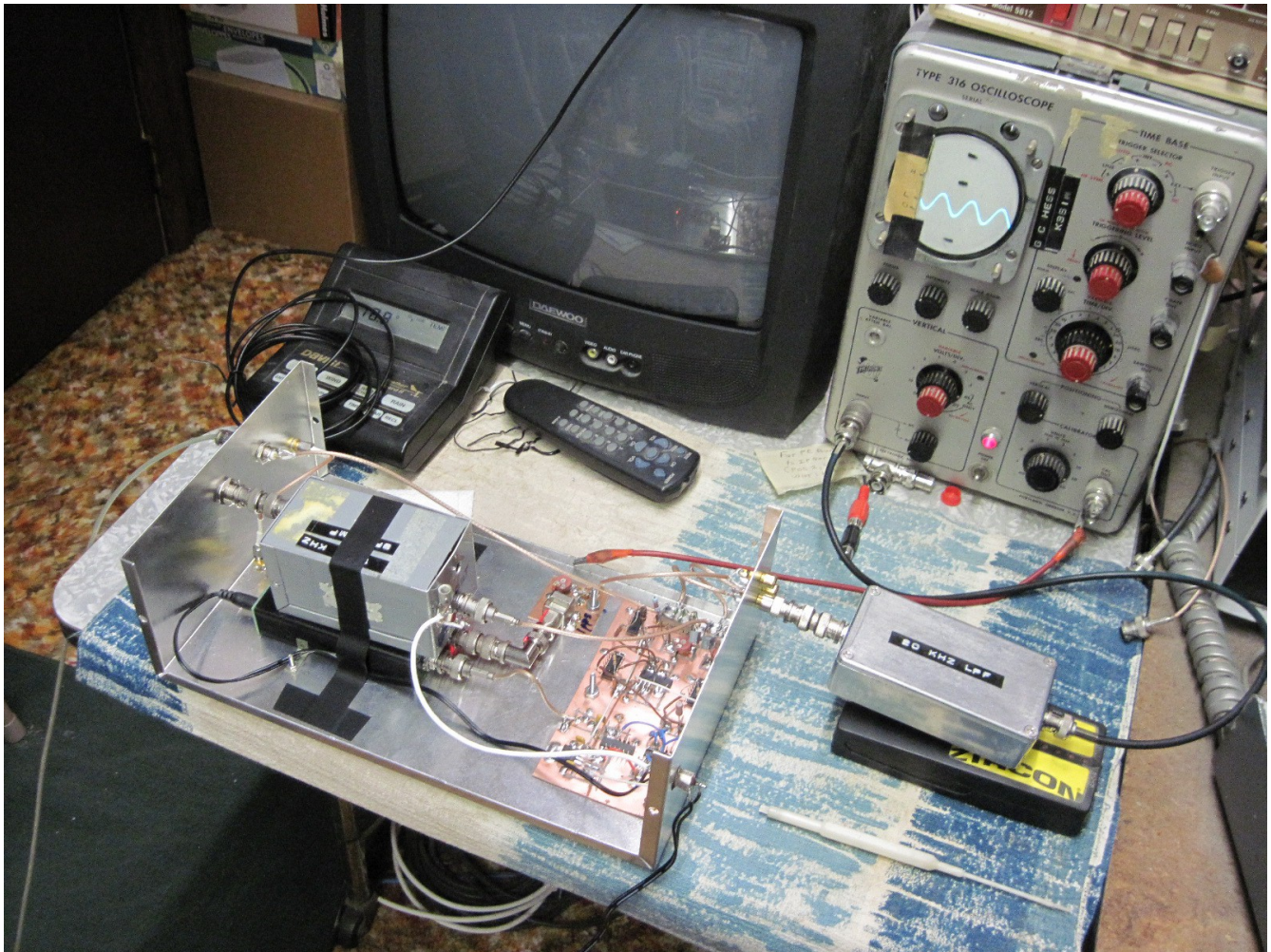
Figure 4 Completed Unit Bench Test: input= -10 dBm from HP Sig Gen @ 185 kHz, downconverted output @ 18.633 kHz (conversion loss including LPF on output < 10 dB); operation for 137.5 kHz input is similar except preselector with gain is included.
