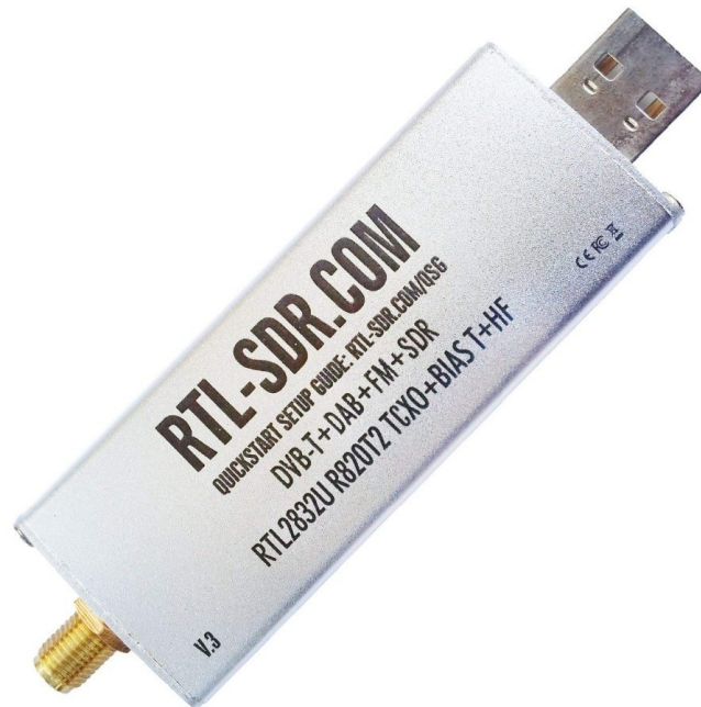
Figure 3: One example of a RTL-SDR receiver stick. They are many varieties and styles on the market.
